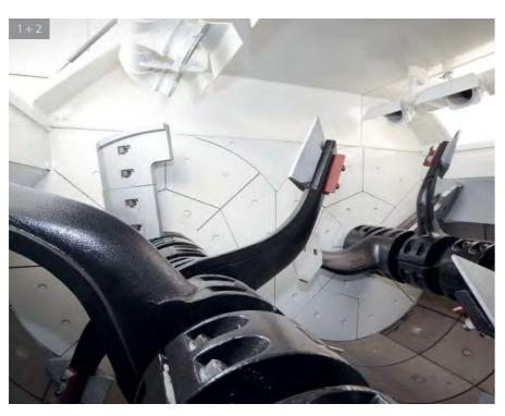
The automatic central lubrication system guarantees a maintenance-free lubrication of all bearings and seals.
