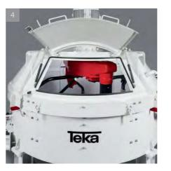
4 | The mixer cover allows for ample space for the material inlets whereby the lifting segments are variable according to customer and batch plant requirements. Large lifting segments ensure optimal access into the mixing area for cleaning and maintenance
