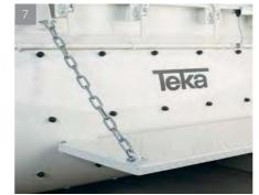
Material inlets are mounted in the area between the mixing shafts. On both sides of the cover there are large openings for cleaning and maintenance.
