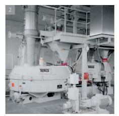
During charging and discharging, each agitator runs at low speed. The agitators are driven by a separate, additional hydraulic power unit.
