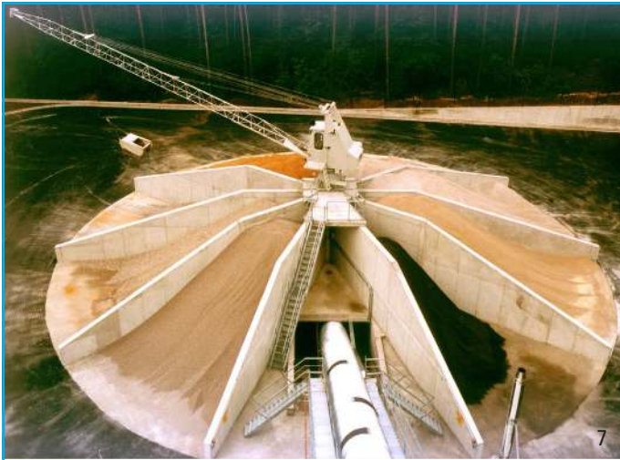
Cover Picture 1: Compact Mortar and Concrete Batching and Mixing Plant MIXOMAT THZ with fully automatic Heavy Duty Scraper THS 60/22.
