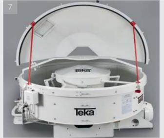
cover, there are no obstructions to impede the arrangement of cleaning segments, inspection doors, material inlets, etc. into the mixing pan.
