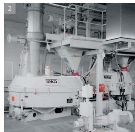
During charging and discharging, each agitator runs at low speed. The agitators are driven by a separate, additional hydraulic power unit.
