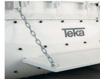
Material inlets are mounted in the area between the mixing shafts. On both sides of the cover there are large openings for cleaning and maintenance.
