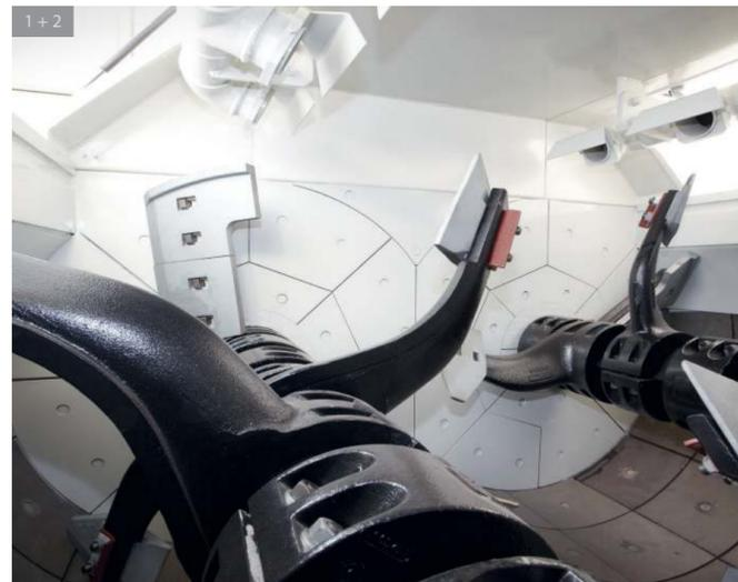
The automatic central lubrication system guarantees a maintenance-free lubrication of all bearings and seals.
